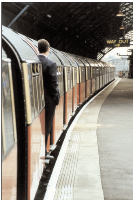
Prior to OPO mirrors and monitors, the Guard was in charge of the platform train interface
