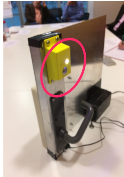
Door access override (figure 3)
